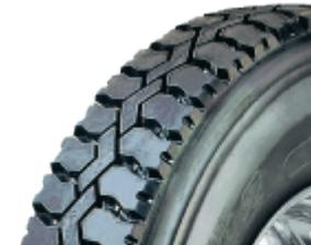
Deep sculpted traction design offering excellent mileage and penetration resistance in both on and off-the-road drive axle applications.
