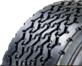
The B857 is an all position tread for on/off highway use offering excellent mileage performance in Wide Base applications.
