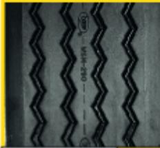
This advanced Wing design gives extra protection so that casing life can be increased, in addition to giving protection against tread edge tearing during cornering and tight manoeuvring.
