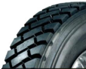
An aggressive drive tread pattern that is designed for severe short haul and off - the - road applications. RLM has a deep skid depth that offers long mileage and increased penetration resistance
